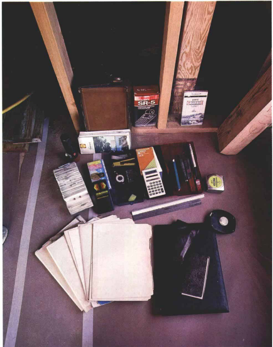
A portable office —Residing inside Gerstel's catalogue case is enough equipment and information to allow him to set up an office anywhere. It includes folders for past, present and future jobs, an adding machine, a company checkbook and a flip file with the names and addresses of business associates. Drawing equipment includes colored and mechanical pencils, gum erasers, architect's scale and a template of typical residential shapes. For remodeling estimates, he carries a stud finder, flashlight and tape measures.
